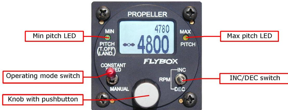
The knob with pushbutton can be rotated (for example to increment or decrement the RPM) or pressed like a pushbutton (for example to enter in the menu or in the various settings).
